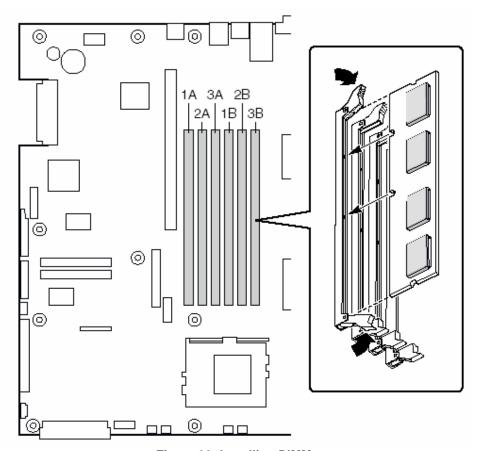
Figure 22: Installing DIMMs
